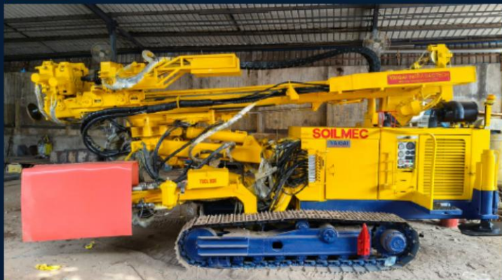
SOILMEC HYDRAULIC CRAWLER RIG
